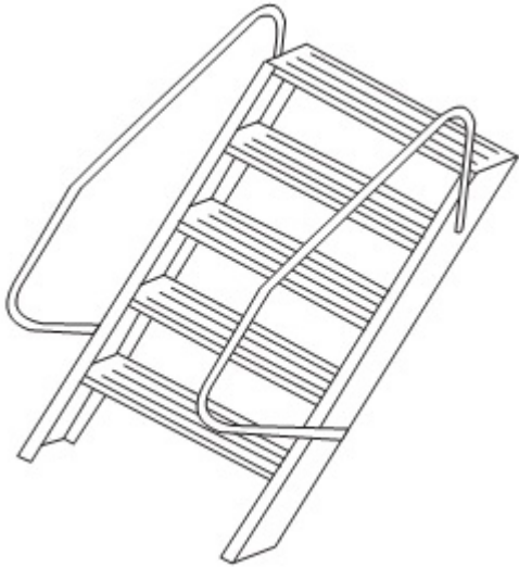
FIGURE 702.3 TYPICAL STAIRCASE LADDER, TYPE C
